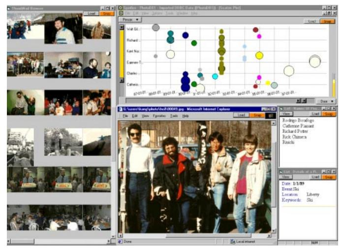
**Figure 6:** Exploring a photo library with Snap. The user has displayed a collection of photos in a thumbnail browser to quickly overview many photos and in a scatter plot to see trends on a time line. These are coordinated to a web browser to display the full-resolution picture of a photo when selected. Additional text views display names of people in the picture and other details.
