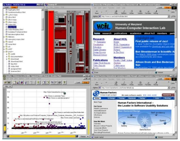
**Figure 5:** This visualization environment for exploring web-site log data was quickly constructed using Snap. The outliner, Treemap, and web browser at the top form a site browser for the HCIL web site. The scatter plot and browser at the bottom display pages that refer readers to the site. This example reveals that Human Factors International referred 110 readers to the HCIL home page that month.
